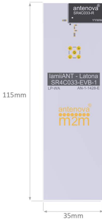
SR4C033-EVB-1 Evaluation Board (For SR4C033-R)
