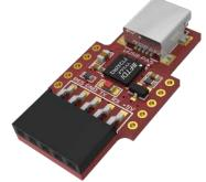
4Duino, or it can be purchased separately. It is the standard programming adaptor used by 4D Systems for other 4D Systems products. The 4D Programming Cable can also be used.
