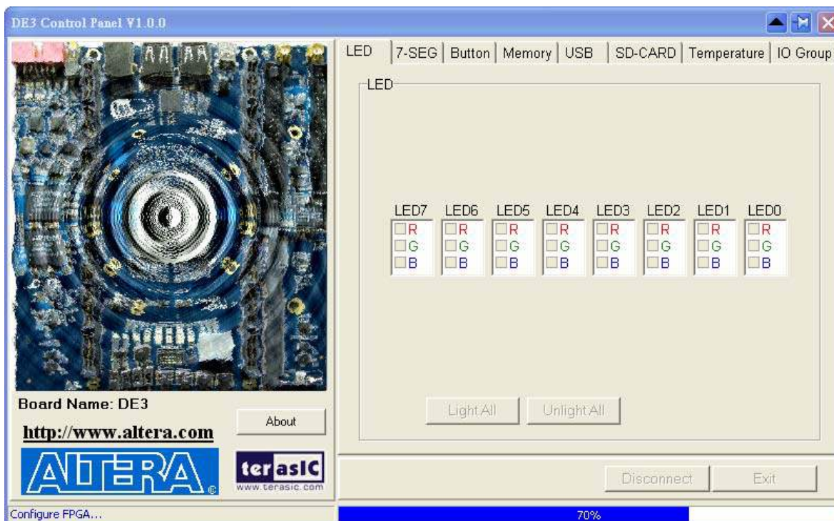
Figure 3.2. Download .sof and .elf files to the DE3 board
