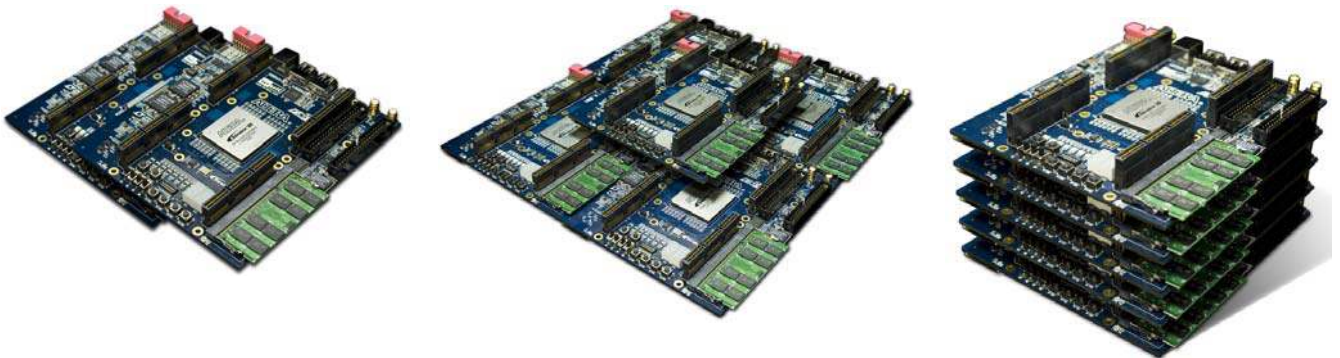
Figure 1.1 The stackable mechanism of the DE3 board
