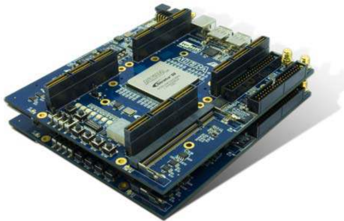
Figure 4.16. The connection of two DE3 boards
