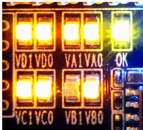
Figure 2.12a. Voltage-Level Indication for I/O Groups Example
