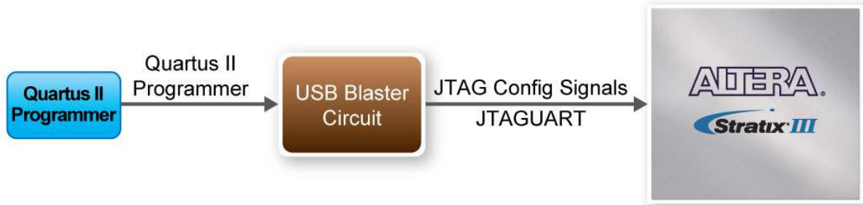
Figure 2.1 The JTAG configuration scheme
