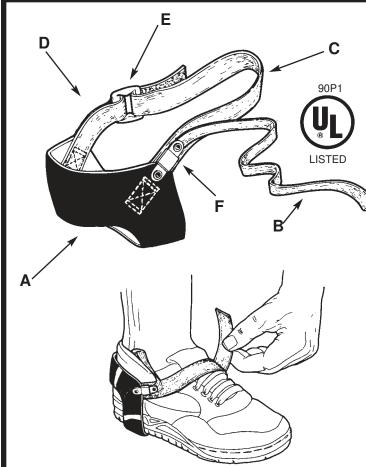
Two heel straps are recommended for reliable grounding and ESD protection, providing ground when one foot is off the floor.
