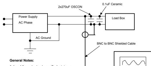
1. Load the outputs at specified minimum output current.
