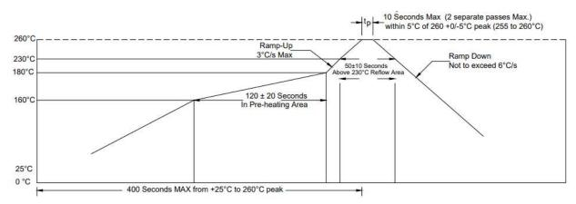
Excessive heating time at high temperature may result in deterioration of the characteristics and may break the crystal unit. For manual rework, heat the lead part at 300°C or lower for 5 seconds or less.
