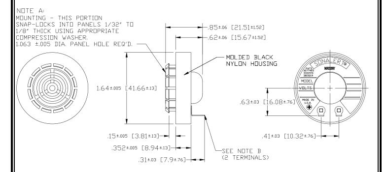
NOTE B: TERMINALS - .016 BRASS, HOT TIN FINISH WITH .076 WIRE HOLE. TERMINAL WILL ACCEPT STANDARD 1/8" QUICK CONNECT
