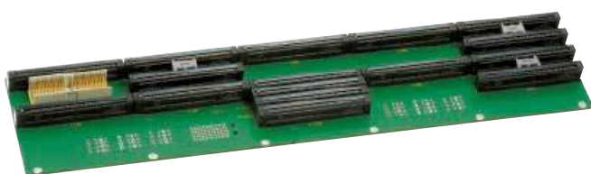
MicroTCA™ backplane with protection blocks
