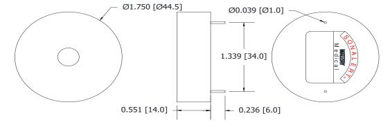
tolerances:  $\begin{array}{c} \pm 0.01 \ [\pm 0.3] \\ \pm 0.005 \ [\pm 0.1] \end{array}$
