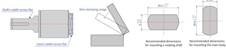
■ The damper's working angle is 110°, as shown below. Rotating the damper beyond this angle will cause damage to the damper. Please ensure that an external stopper is in place. The working angle is based on the width across flat for fixing, located towards the rear end of the main body. The position where the rotation is complete is at 90° with respect to the width across flat.
