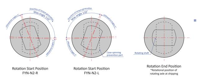
The direction in which torque is generated varies according to the model.
