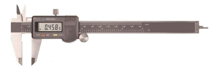
Thumb wheel adjustment for easy to dial in measurements.
