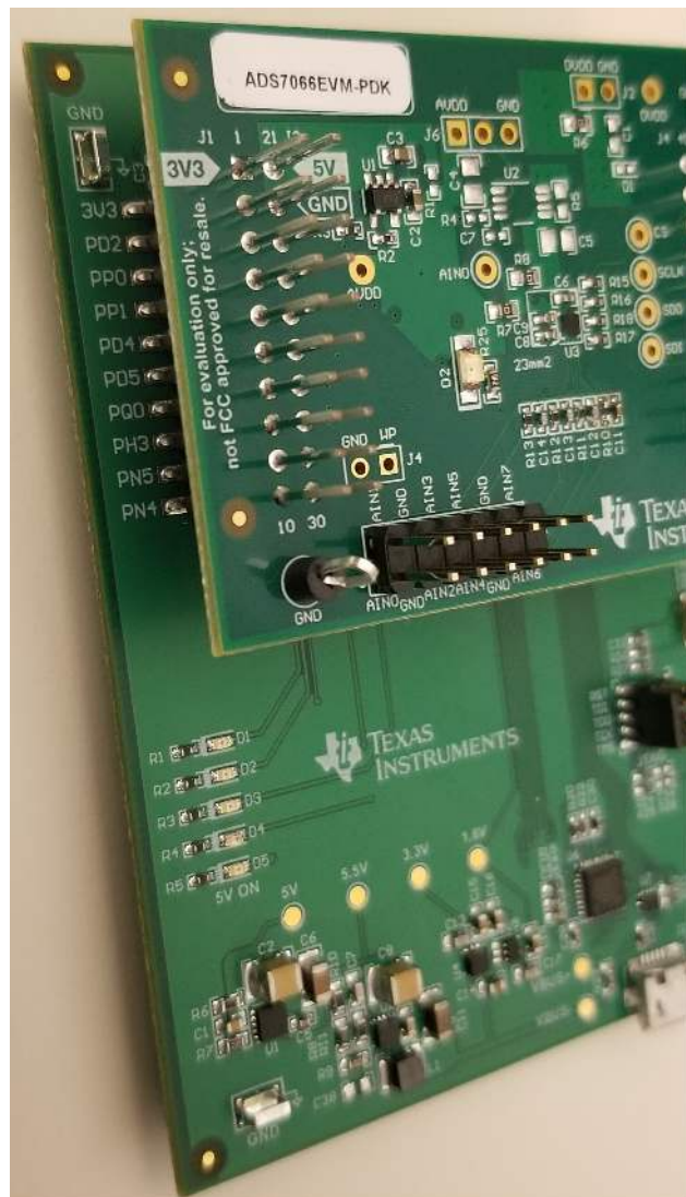
Figure 4. ADS7066EVM Lined up With PAMBoard (Left View)
