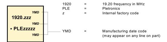
The actual part number is TCD4025-19.20M where the model number "025" is the specification number the part is made to. This is not included in the part marking. This is included on the label on the Tape and Reel.
