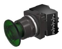
30mm BlackMax, Epoxy Coated Corrosion Resistant Complete Metal Unit Illuminated Twist-to-Release Transformer type, 240V AC Incandescent Lamp Mushroom Head Cap Small 1.79" (45 mm) Plastic Cap, Green 2 Position Maintained, Twist-to-Release with 1 N.O. - 1 N.C. Heavy Duty Contacts, A600/P600 UL Listed, CSA Certified NEMA 1,3,3R,4,4X,12,13 & Automotive Standards
