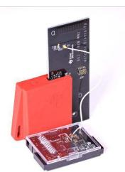
Antenna board #9 has been snapped out from the CC-Antenna-DK2 panel and is connected to a SensorTag via the JSC to JSC cable<sup>2</sup>.
