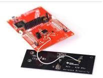
Antenna board #8 has been snapped out from the CC-Antenna-DK2 panel and is connected to a LaunchPad via the JSC to JSC cable<sup>2</sup>.
