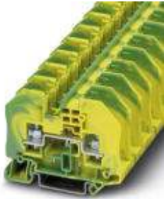
Ground terminal block with bolt connection, cross section 0.1 - 2.5 mm 2 , AWG: 26 - 14, width 12.3 mm, color: Green-yellow
