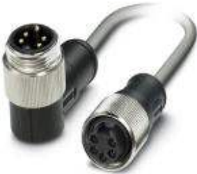
Bus system cable, DeviceNet, 5-position, PUR halogen-free, Gray RAL 7001, Plug angled 7/8"-16UNF, on Socket straight 7/8"-16UNF, Cable length: 15 m
