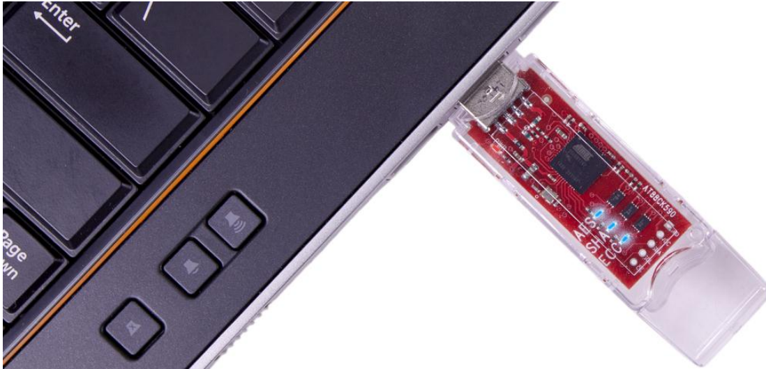
Figure 2. Kit Powered Through USB Port
