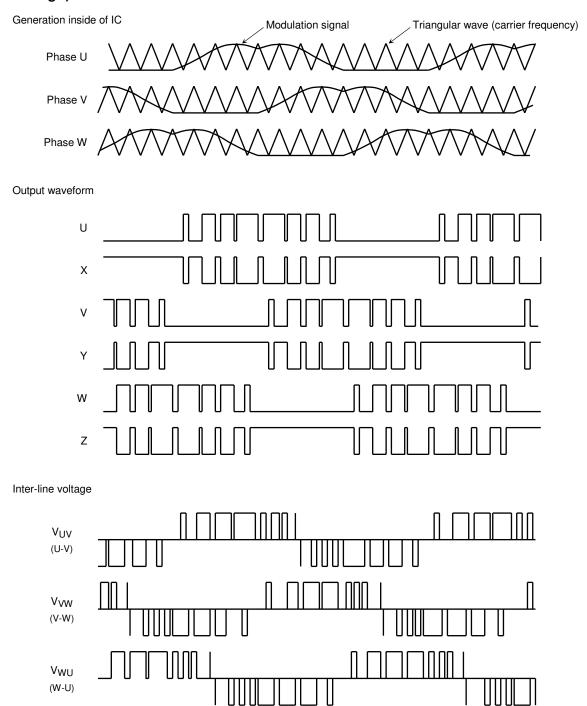
When driven by a sine wave, the motor is accelerated or decelerated according to the ON duty of  $T_{ONU}$  as the amplitude of the modulation symbol changes according to voltage  $V_e$ . (See the diagram of the modulation ratio on page 14.)
