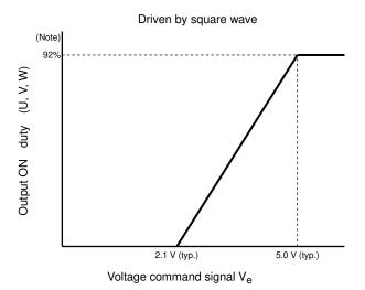
Note: Output ON time is decreased by the dead time (carrier cycle  $\times$  92% –  $T_d \times 2$ )
