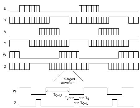
To stabilize the bootstrap voltage, the lower outputs  $(X,\,Y,\,\text{and}\,Z)$  are always turned on at the carrier cycle even during off time. At that time, the upper outputs  $(U,\,V,\,\text{and}\,W)$  are assigned dead time and turned off at the timing when the lower outputs are turned on.  $(T_d\,\text{varies}\,\text{with input}\,V_{e.})$
