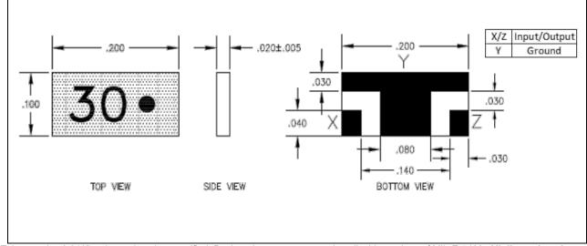
Tolerance is  $\pm 0.010$ ", unless otherwise specified. Designed to meet or exceed applicable portions of MIL-E-5400. All dimensions in inches.
