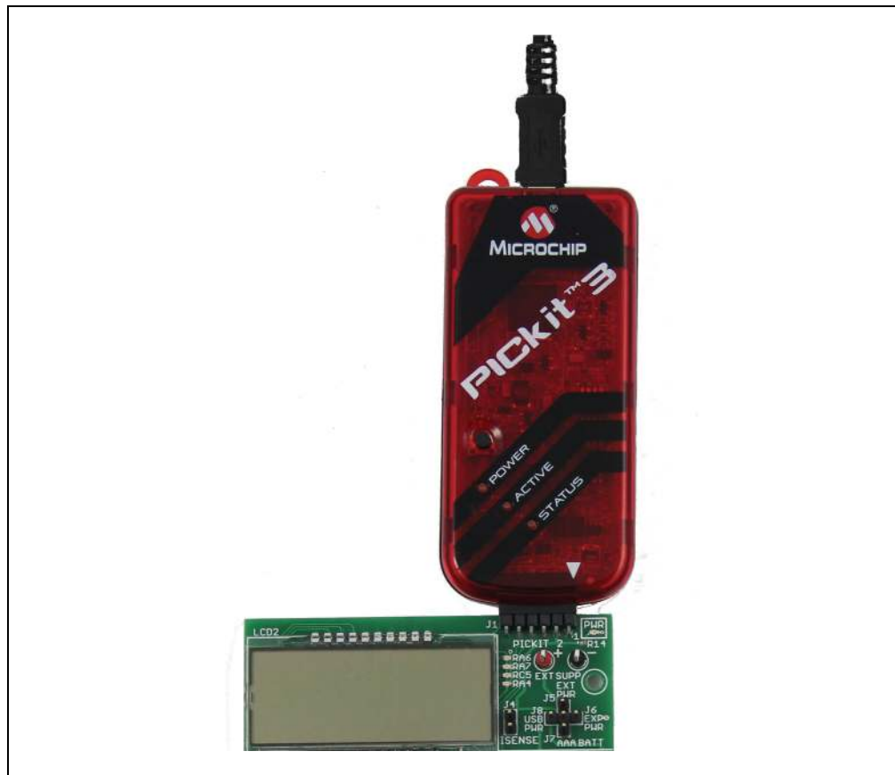
FIGURE 2-2: POWERING FROM PICKit™ 3
