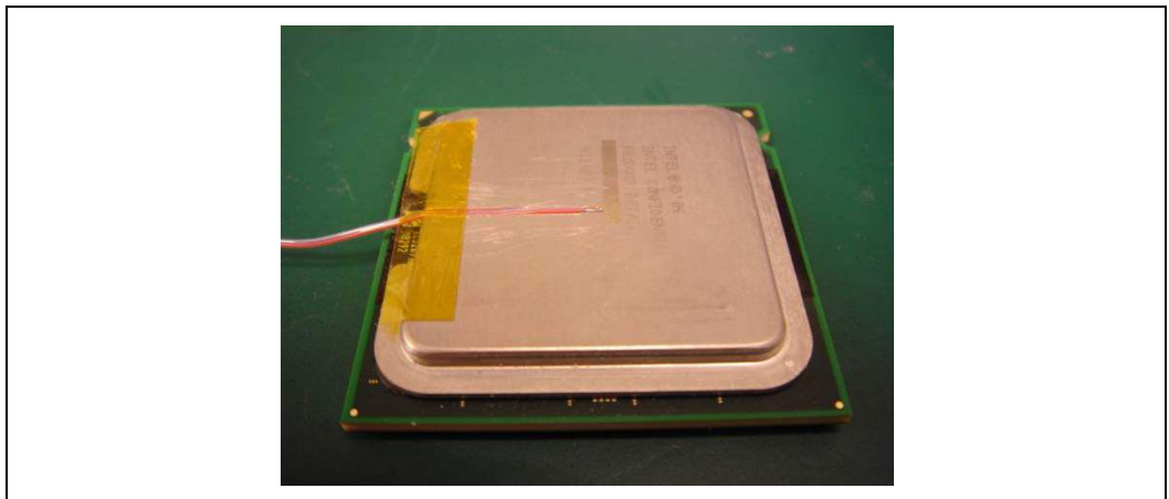
Figure 7-18. Securing Thermocouple Wires with Kapton* Tape Prior to Attach
