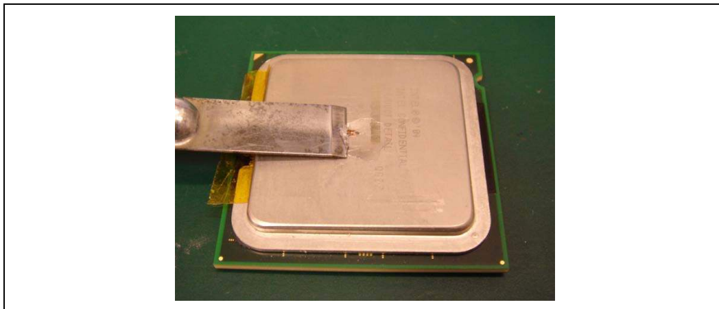
Figure 7-35. Removing Excess Adhesive from IHS
