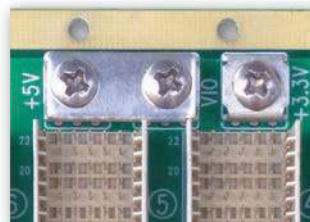
V I/O busbar
