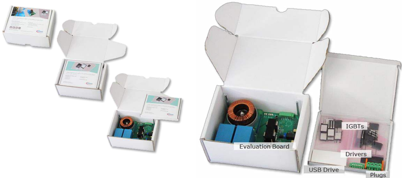
Figure 2 Scope of delivery: evaluation board, spare parts and USB drive with documentation
