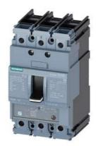
circuit breaker 3VA5 UL frame 125 breaking capacity class S 25kA @ 480 V 3-pole, line protection TM240, ATAM, In=80A overload protection Ir=64A ...80A short-circuit protection Ii=5...10 x In cable connection on both sides
