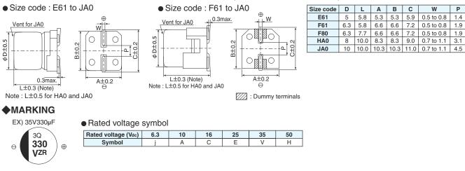
Applying voltage over the rated voltages causes the capacitors to have short lifetime. Besides, applying voltage over the specified surge voltages may cause to have short circuit failure. A protection circuit should be used if applied voltage will exceed the rated voltages.
