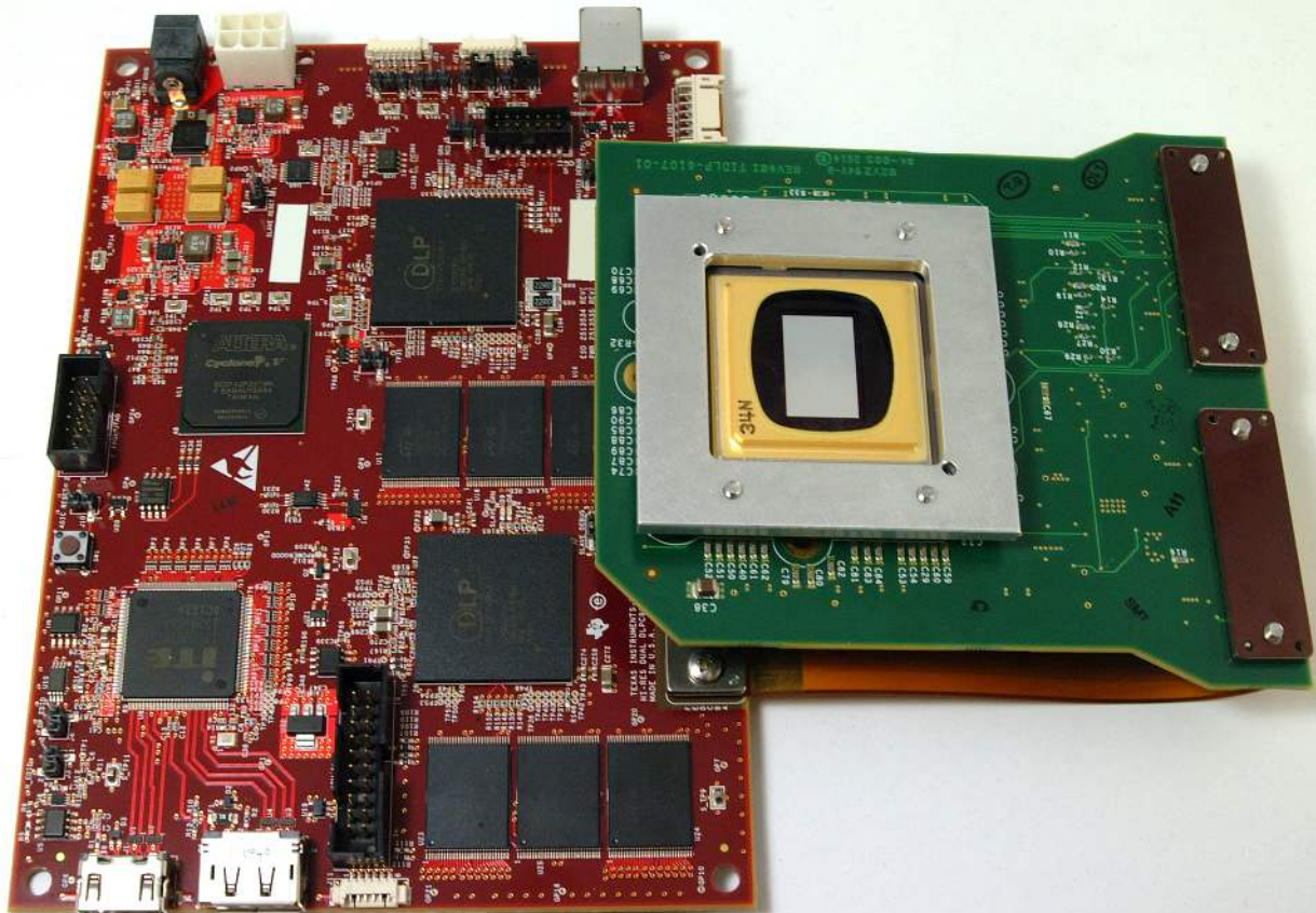
Figure 2. DLP LightCrafter 9000 Evaluation Module
