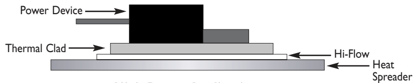
High Power Application Hi-Flow with Thermal Clad
