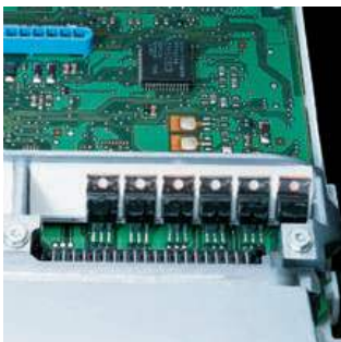
A common Sil-Pad application includes TO-220 transistors mounted in a row on a heat rail.
