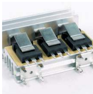
Choose a Sil-Pad that optimizes thermal performance for our mounting method — screw, clip, spring, bar, and so on.
