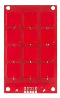
The keypad has 5 lines that need to be connected to your microcontroller, including the power lines, the IRQ line and the I<sup>2</sup>C lines.
