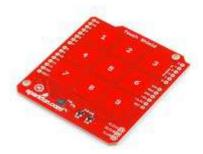
The shield connects directly to the 3.3V pin on the Arduino. There is no onboard voltage regulation on the VCC line, so keep that in mind if you intend to use this with a 5V Arduino Pro board. However, there is an onboard logic level converter to step down 5V levels to the 3.3V for the sensor's I<sup>2</sup>C lines.
