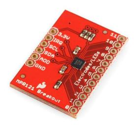
The breakout board has 4 pins that need to be connected to your microcontroller at a minimum to get communication going: the power lines and the I<sup>2</sup>C lines. However, for our example, we are going to be also connecting the IRQ pin to more easily detect a change on one of the electrodes.
