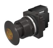
30mm BlackMax, Epoxy Coated Corrosion Resistant Complete Metal Unit Illuminated Push-Pull Operator Transformer type, 120V AC Incandescent Lamp Mushroom Head Cap Small 1 3/4" (44.5 mm) Metal, Black with Amber Lens 3 Position Pull-Momentary/Push-Maintained UL Listed, CSA Certified NEMA 1,3,3R,4,4X,12,13 & Automotive Standards
