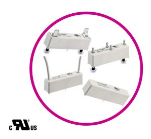
The DB(UL) series is a UL\* approved very high isolation voltages (up to 10kV) are achieved through the use of high vacuum reed switches with either rhodium or tungsten contacts and make these relays suitable for high reliability applications, such as cardiac defibrillators, test equipment and high voltage power supplies.
