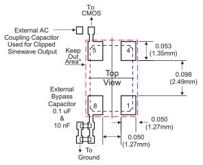
\* Do not route any traces in the keep out area. It is recommended that the next layer under the keep out area is to be ground plane.
