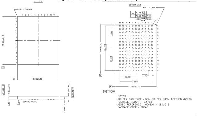
Figure 10. 165-Ball FBGA (13 X 15 X 1.4 mm)
