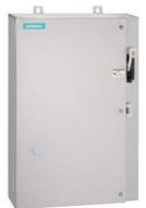
Non-reversing motor starter Size 4 Three phase full voltage Solid-state overload relay OLRelay amp range 50-200A 550/575-600 50/60HZ coil Combination type 200A fusible disconnect 200A/600V fuse clip Encl NEMA type 4X 304 S-steel Water/dust tight noncorrosive Standard width enclosure
