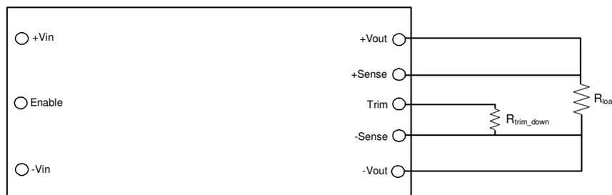
Figure 16. Trim DOWN circuit configuration
