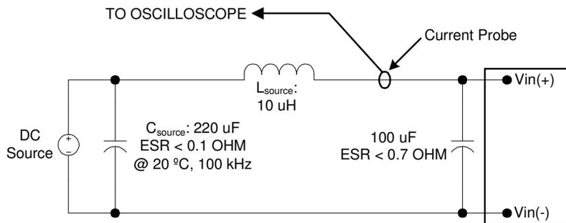
Note: Measure input reflected-ripple current with a simulated source inductance ( $L_{test}$ ) of 10  $\mu\text{H}$ . Capacitor  $C_s$  offsets possible source impedance.
