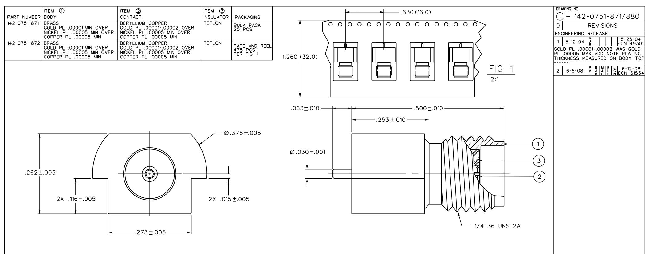
NOTE: TO INSURE THAT NO DAMAGE TO THE CONNECTOR-TO-BOARD SOLDER JOINT OCCURS, IT IS RECOMMENDED THAT A WRENCH BE USED TO SECURE THE CONNECTOR BODY AND THAT A MAXIMUM OF 8 INCH-POUNDS OF TORQUE BE APPLIED TO THE MATING CONNECTOR COUPLING NUT.
