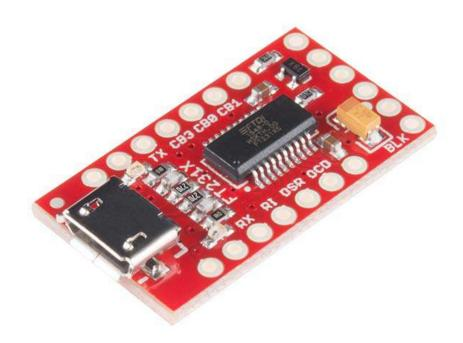
Introducing the 3.3V SparkFun FT231X Breakout board, complete with the full UART hardware handshake feature! The pin-out of this board matches the FTDI cable to work with official Arduino and cloned 3.3V Arduino boards. It can also be used for general serial applications.
