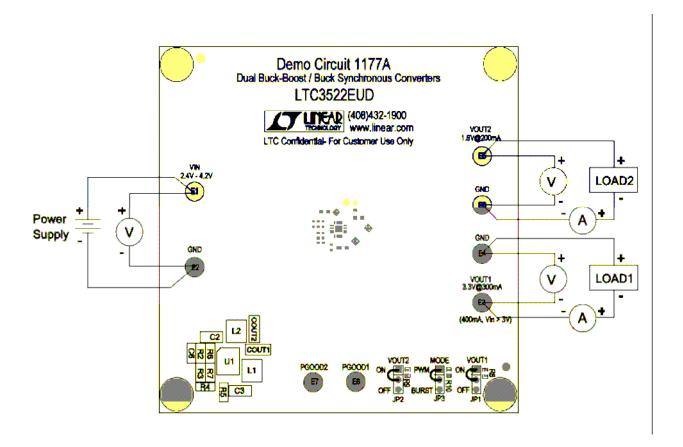
Figure 1. Proper Measurement Equipment Setup
