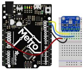
The final results should resemble the illustration above, showing an Adafruit Metro development board.
