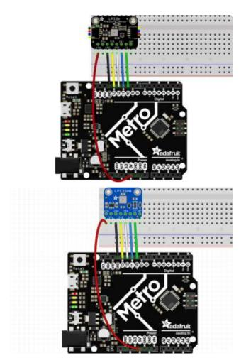
Connect Vin to the power supply, 3V or 5V is fine. Use the same voltage that the microcontroller logic is based off of Connect GND to common power/data ground
