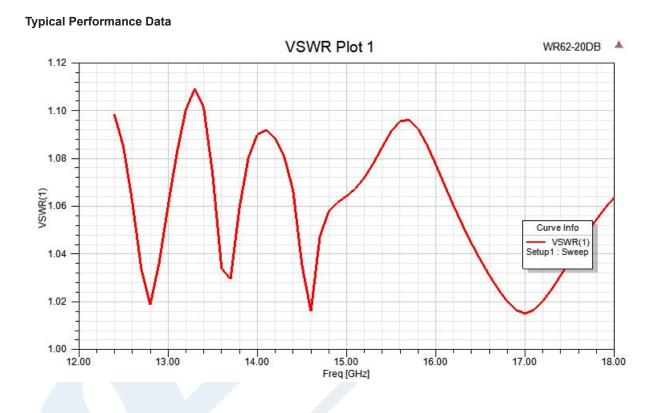
Click the following link (or enter part number in "SEARCH" on website) to obtain additional part information including price, inventory and certifications: WR-62 Standard Gain Horn with 20 dBi gain, End Launch SMA Female connector PEWAN062-20ELSF
