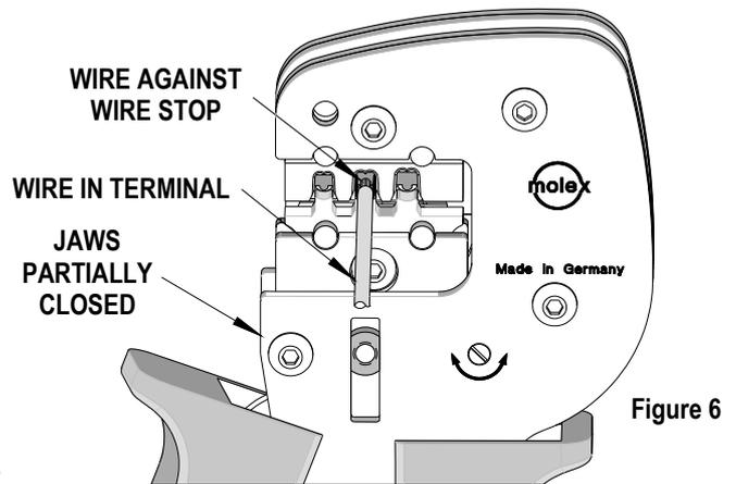
6. Turn the Locator Lock Latch up to lock. Make sure that the terminal is visually centered over the punch.
