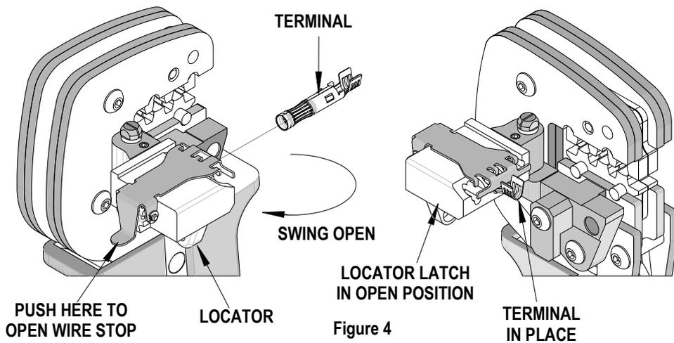
3. Swing the terminal locator away from the crimp tool shown in Figure 4. Some terminals with large conductor grips may interfere with the crimp tooling when swinging the locator into position. The terminal must then be loaded into the locator in the closed/crimp position. See Figure 5.
