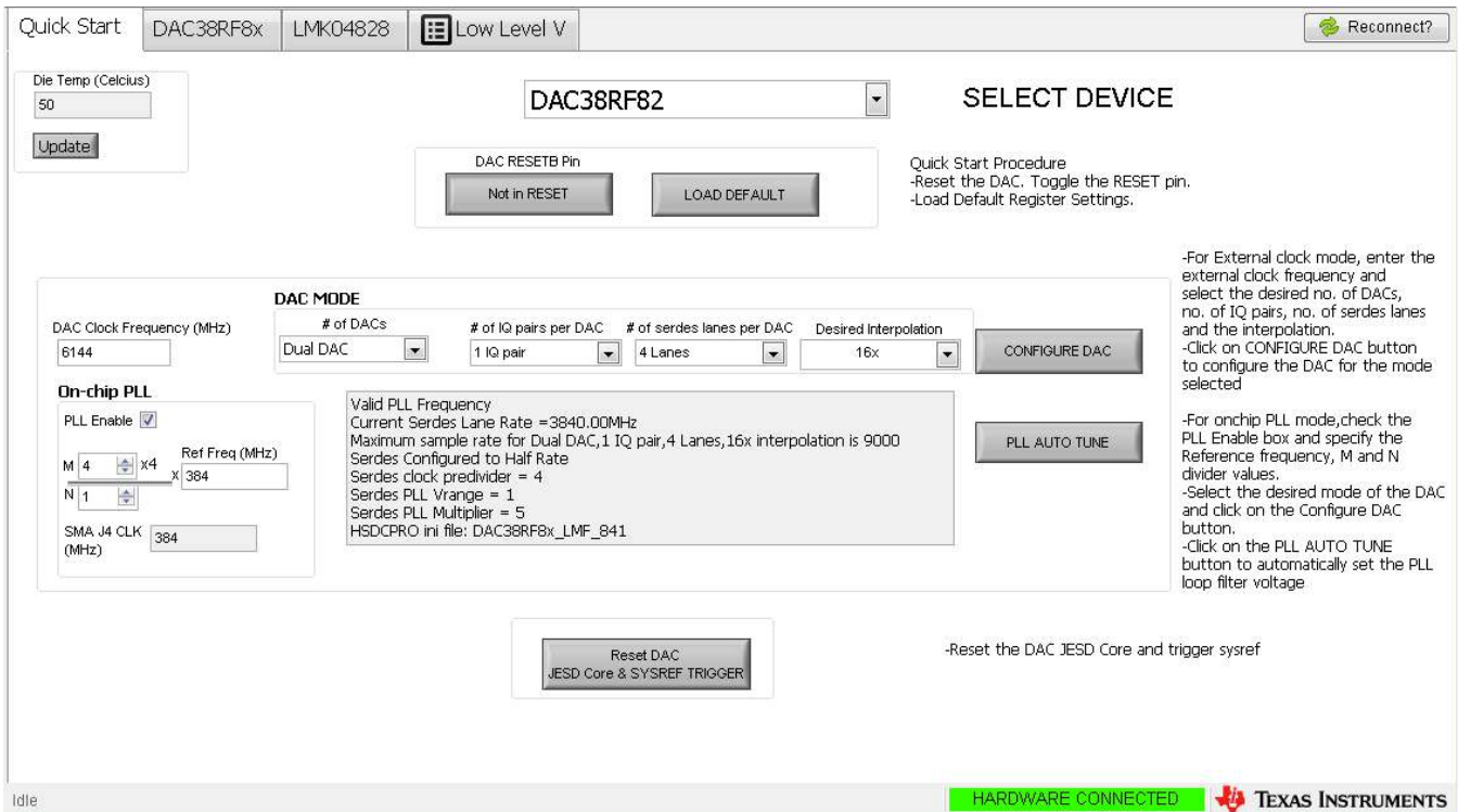
Figure 8. DAC38RF8xEVM GUI Quick Start Page Configured for On-Chip PLL Mode
