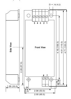
\* Unscrew DIN connector for chassis mounting.
