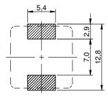
no vias and sensitive traces underneath the component Scale - 2:
