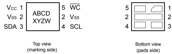
Figure 2. 5-pin package connection
