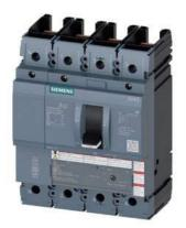
circuit breaker 3VA5 UL frame 250 breaking capacity class M 35kA @ 480 V 4-pole, line protection TM240, ATAM, In=100A overload protection Ir=80A…100A short-circuit protection li=5…10 x In N conductor protection 100% without connection
