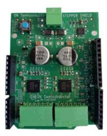
The Dual Stepper Motor Driver Shield Evaluation Board evaluates the AMIS30543, a microstepping stepper motor driver for bipolar stepper motors. It has an on chip voltage regulator, reset output and watchdog reset able to supply peripheral devices. The chip is connected through IO pins and a SPI interface with an external microcontroller that is regulated through the PCA9655E's 16 bits of General Purpose parallel Input and Output (GPIO) expansion.
