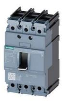
circuit breaker 3VA5 UL frame 125 breaking capacity class S 25kA @ 480 V 3-pole, line protection TM210, FTFM, In=15A overload protection Ir=15A fixed short-circuit protection Ii=20 x In UL489 SB (naval), 50 deg. cel. cable connection on both sides
