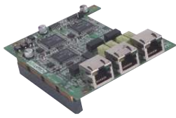
MIO-6250 3 x 10/100 Mbps with Bypass Ethernet Ports
