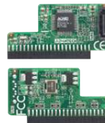
PCM-233C IDE (44-pin) to SATA Converter Module
