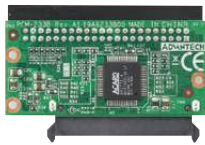
PCM-233B IDE (44-pin) to SATA Converter Module
