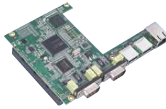
MIO-6260 Multi I/O Module with 1 Ethernet, 2 COM, 4 USB
