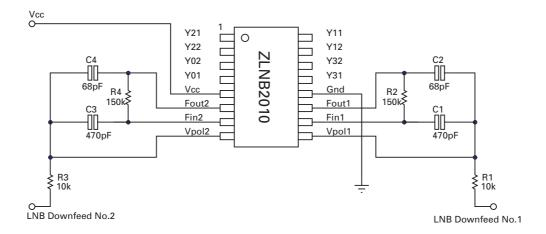
The following circuit shows the additional components that will be used for polarisation mode and 22kHz tone detection in typical ZLNB2006/9 application
